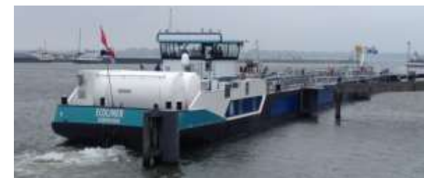
LNG-fuelled type C tanker EcoLiner developed by DAMEN within the LNG Masterplan for Rhine-Main-Danube project (2013-2015) © DAMEN
